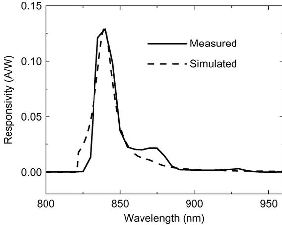
Fig. 10. Comparison between measured and estimated responsivities of the NIR quantum well stack, for an applied bias of 1 V and temperature of 10 K.
