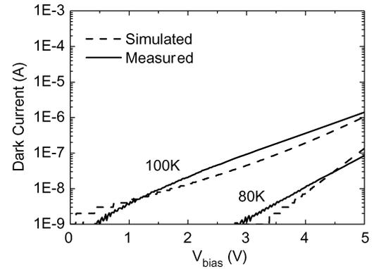
Fig. 4. Comparison between theoretically predicted and measured dark current values for MWIR quantum well stacks at temperatures of 100 and 80 K.
