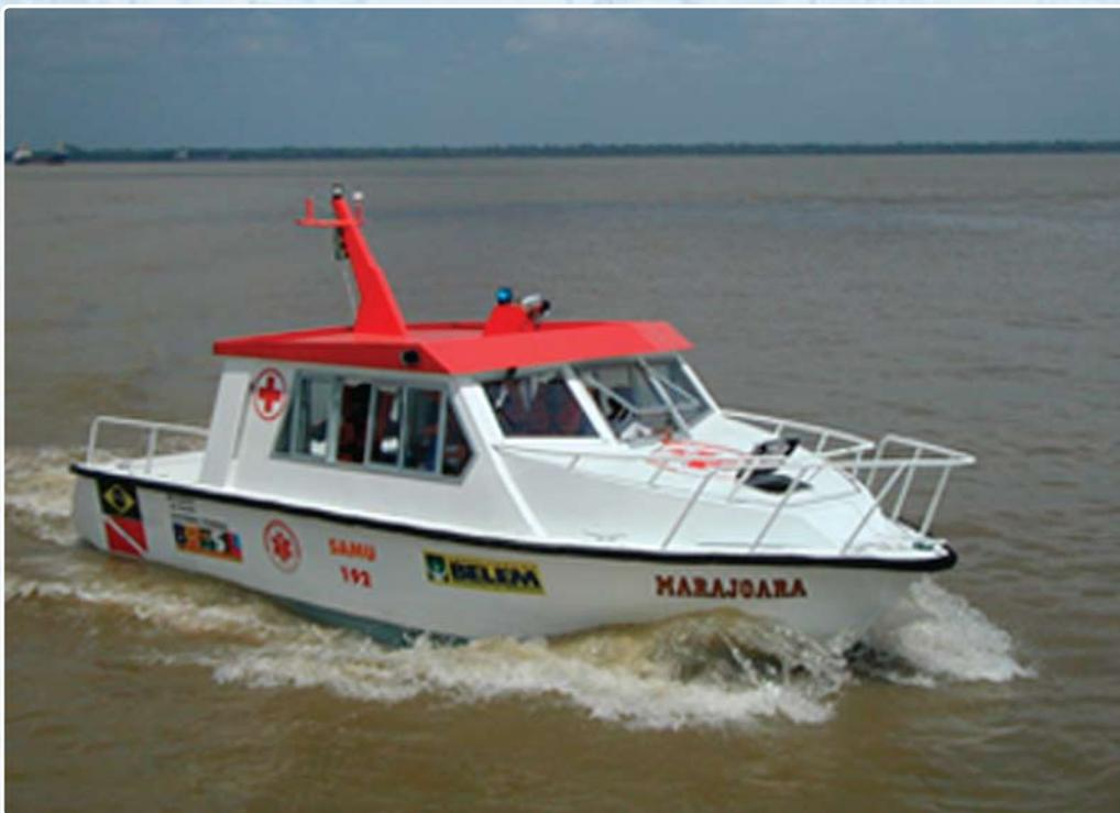
The Ambulance Craft - LAM, built at Val-de-Cães Naval Base, located in Belém, is a versatile boat, suitable for fast removal of wounded on riverine environment. Made of naval aluminium alloy, LAM transports up to two patients and a crew of four
